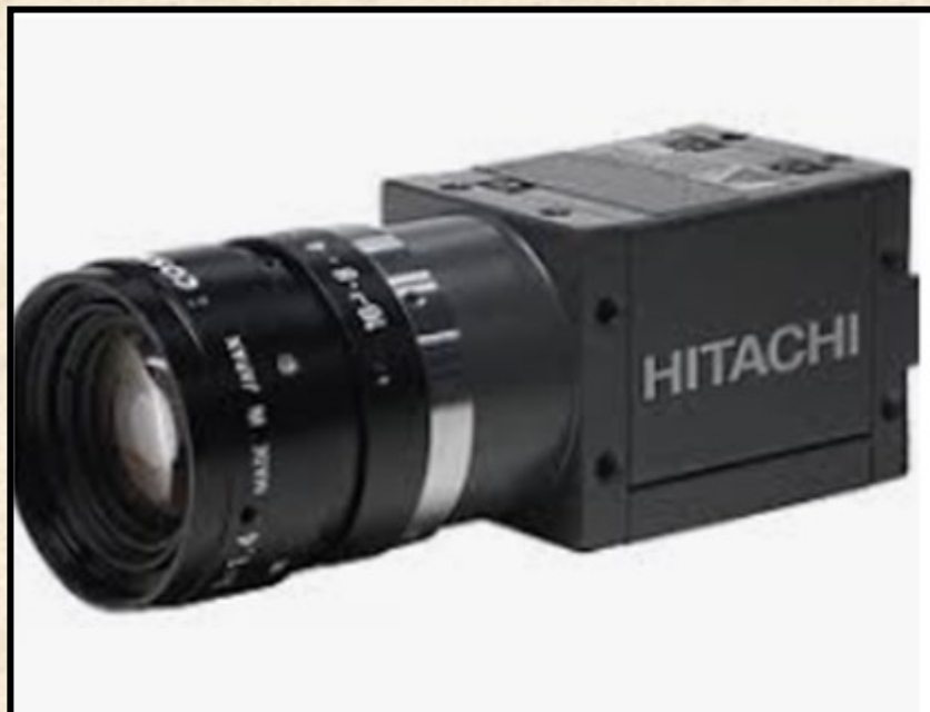
Fig.1 A Charge-coupled device camera
